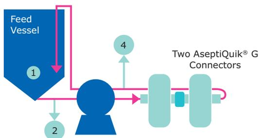
**Figure 6:** Schematic of Lynx® and AseptiQuik® G Connectors Setup used during solvent recirculation
