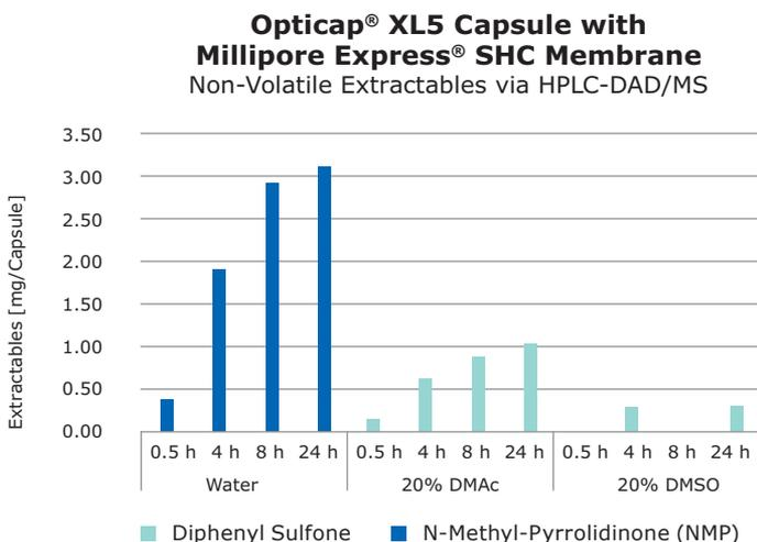
**Figure 3:** Non-volatile extractables for Opticap® XL5 Capsules with Millipore Express® SHC membrane
