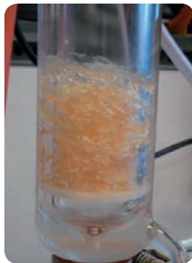
Figure 4. Wax-like, amorphous DOPE in comparison to free flowing powder DOPE.
