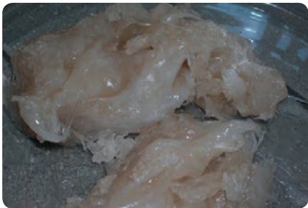
Figure 4. Wax-like, amorphous DOPE in comparison to free flowing powder DOPE.
